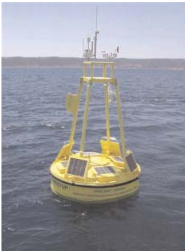
In situ moored-buoy automatic oceanographic and meteorological station, Middle Adriatic Sea, Institut of Oceanography and Fisheries, Split, Croatia
