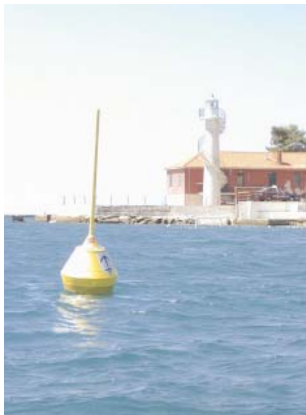
In situ moored-buoy automatic station for sea temperature measurement Umag, MHS, Croatia
