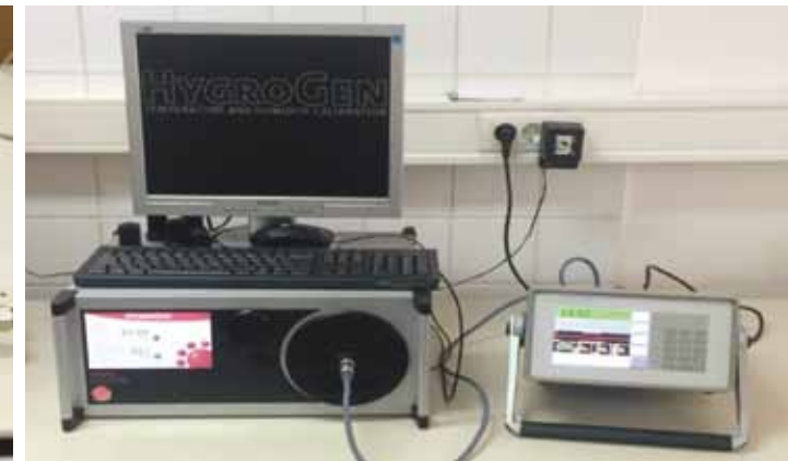
The reference system for the calibration of instruments for measuring relative air humidity (on the left) and mass flow rate (on the right)
