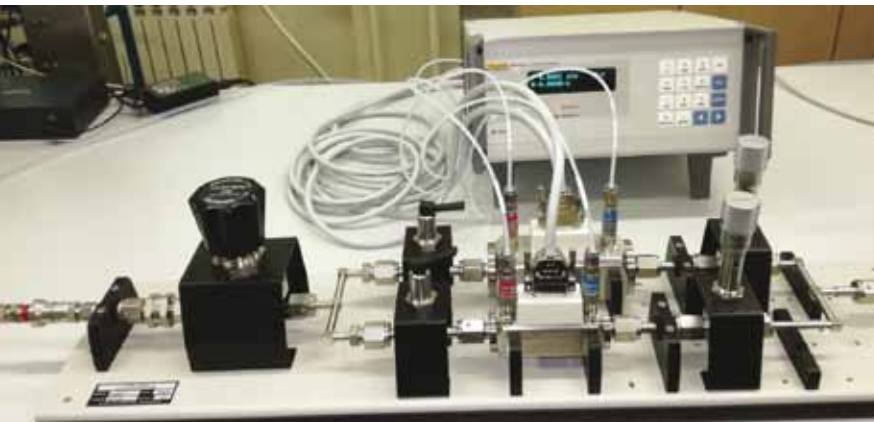
The reference system for the calibration of instruments for measuring relative air humidity (on the left) and mass flow rate (on the right)
